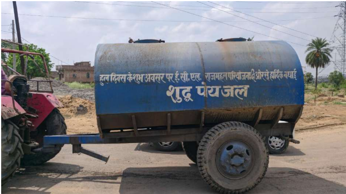
Photograph-5(c) Water tankers for distribution of potable water to nearby villages
